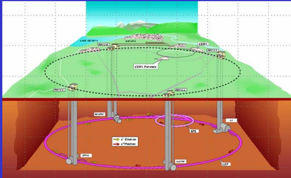
27 km long LHC tunnel filled with SC magnets. Beam loss monitoring by 3700 ionization chambers, which are replaced in experimental area with diamond sensors.
