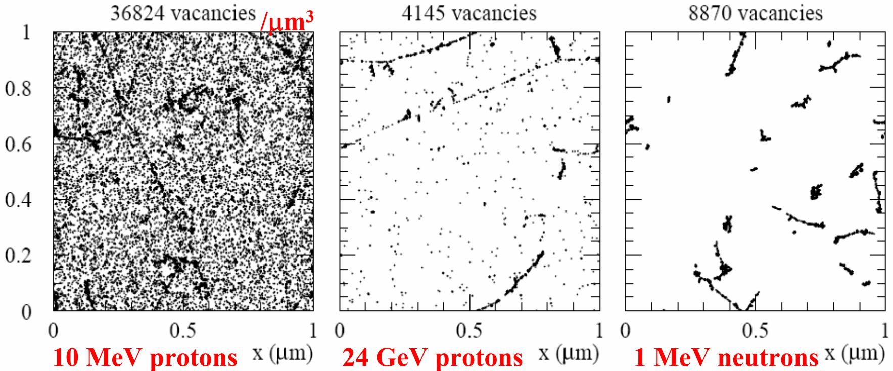
Conclusion: most dangerous beams are low energy charged particles (due to Rutherford scattering)
