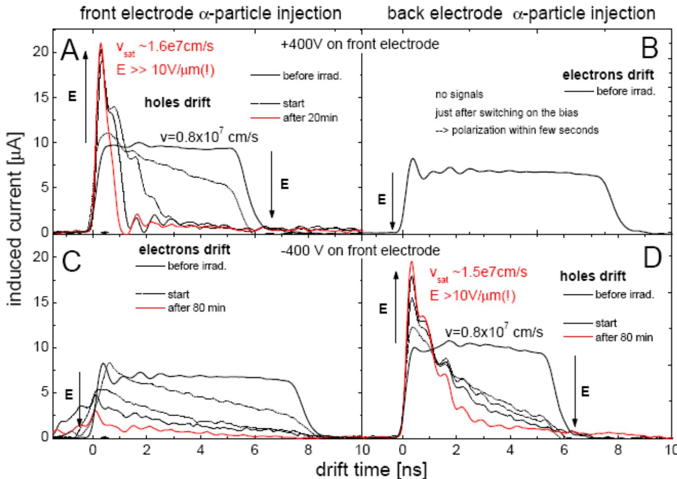
Similar effect observed in CdTe and irradiated cryo Si (reverse biased)
