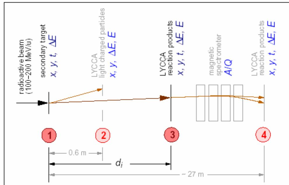
1. Target (Be, Au..), position (DSSD) and time start (CVD diamond)
