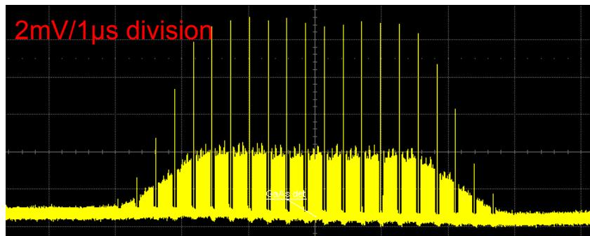
Signal constant over duration of heatload chopper pulse.
