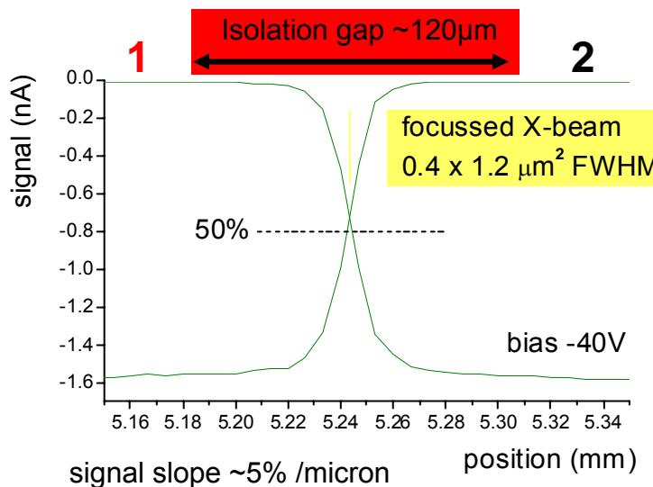
For small beam ( $\sim\mu\text{m}$ ), crossover response is convolution of photoelectron thermalization range ( $\sim 1\mu\text{m}$ ) and lateral charge diffusion ( $5\sim 50\mu\text{m}$ ) which occurs during drift of  $e^-$ ,  $h^+$  charge carriers
