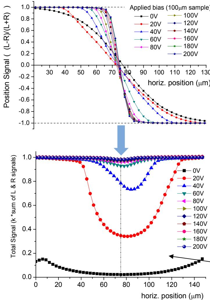
nb. low frequency Electrometer current measurements
