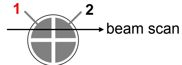
For large beam ( $> 50\mu\text{m}$ ), quadrant 'crossover response' is  $\sim$  line integral over the beam intensity profile
