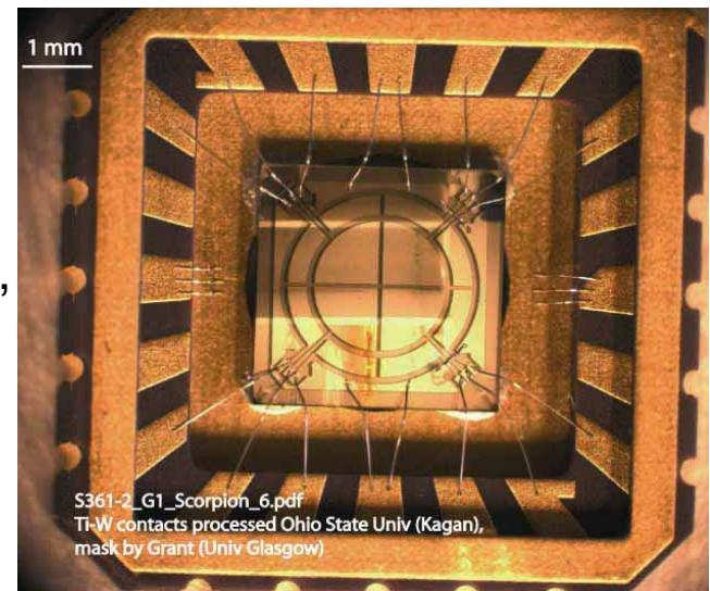
Packaged device tests ID09B
