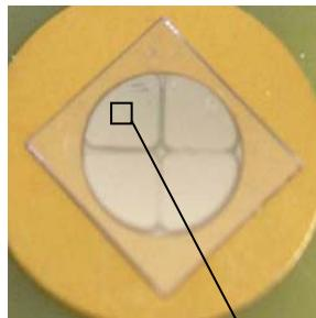
50 $\mu\text{m}$  thick sample, bias 50V, 50nm sputtered Al-Al contacts (GSI Target Lab).
