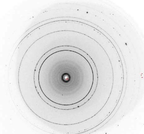
Scattered beam 'powder diffraction' rings arising from the  $\sim 10\mu$ m random orientation grains of the polycrystalline diamond plate
