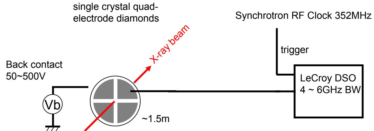
ID21: focused X-ray beam  $\sim 0.5 \times 0.1 \mu\text{m}^2$  and  $\sim 10^2 \text{ ph/pulse}$  at 6keV
