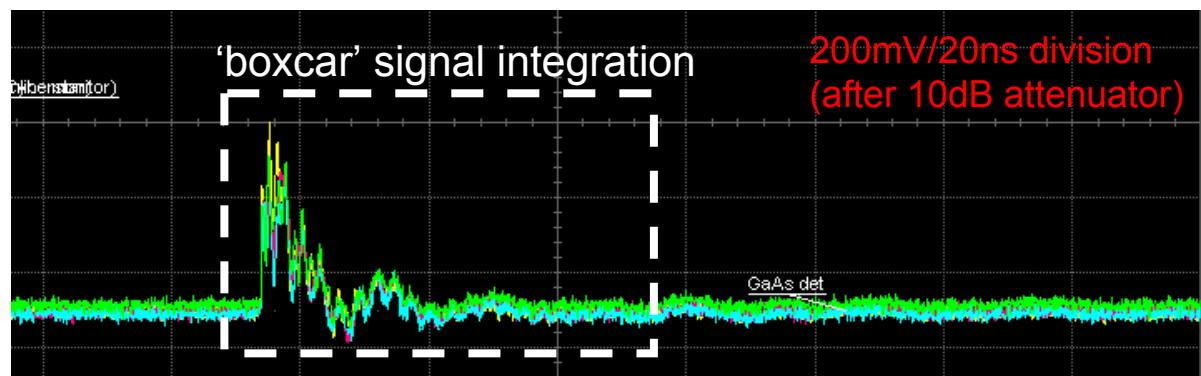
*Very poor circuit layout & cabling of diamond support → signal 'bounce'*
