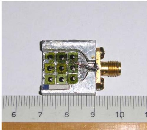
*Nine diamond detectors connected in parallel and tested under  $\alpha$  particles irradiation*
