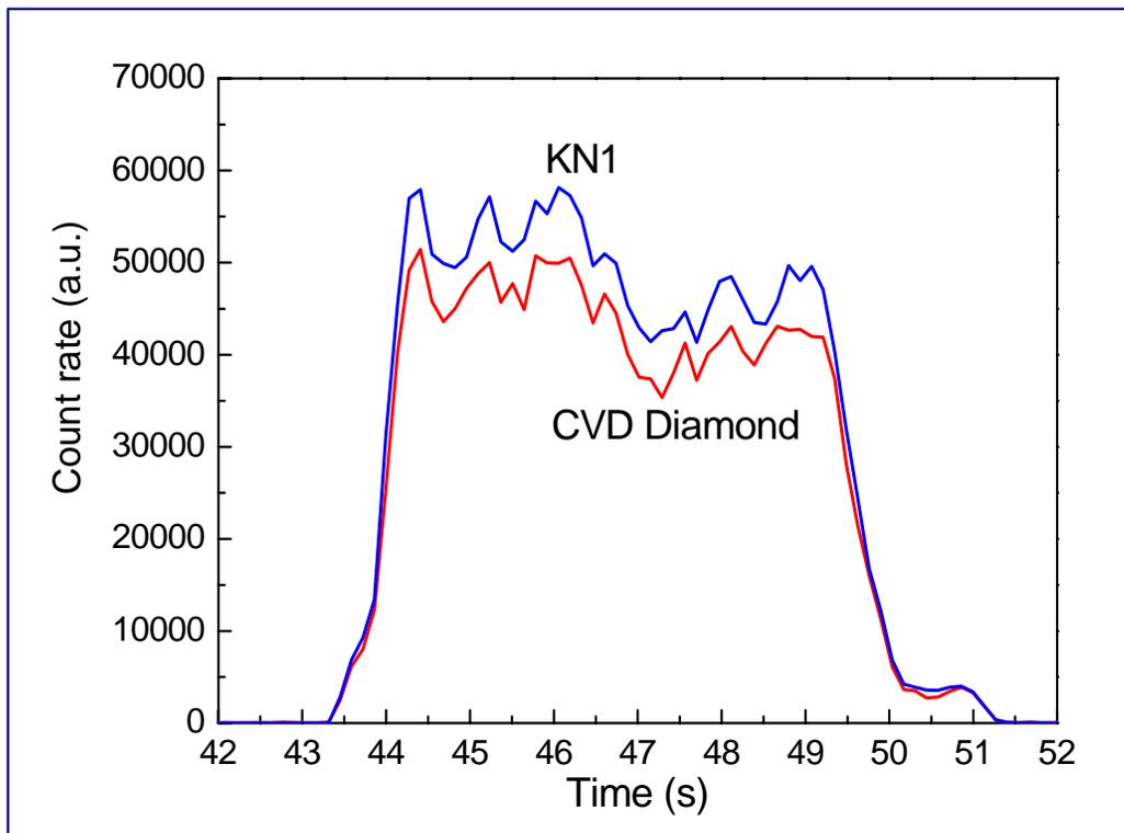
*Comparison of time dependent neutron emission measured by a CVD diamond and KN1 system during a JET pulse.*
