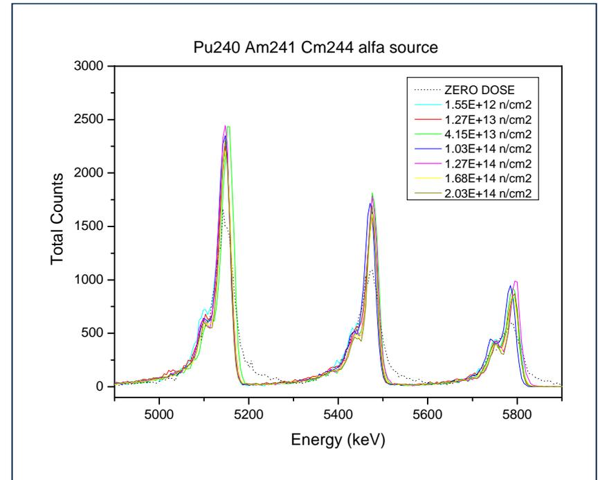
$\alpha$  particles spectra after sequential 14 MeV fast neutrons irradiations
