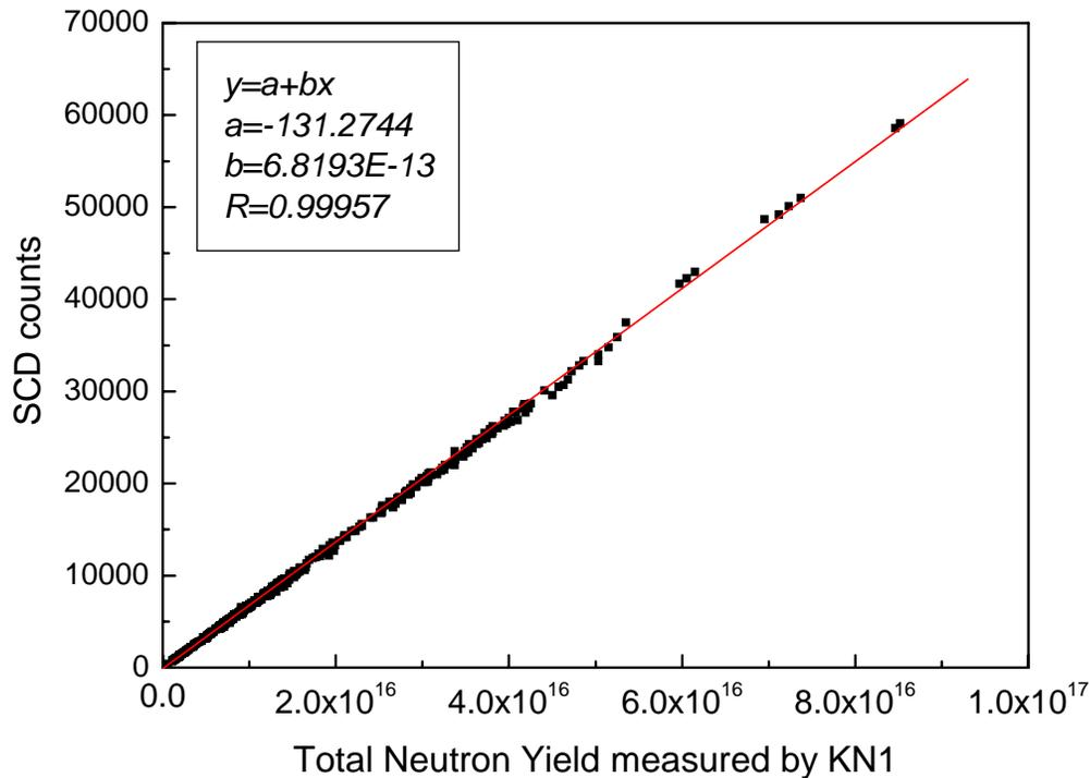
**Comparison between CVD diamond detectors and KN1 JET acquisition system (official monitor) over 400 JET shots.**
