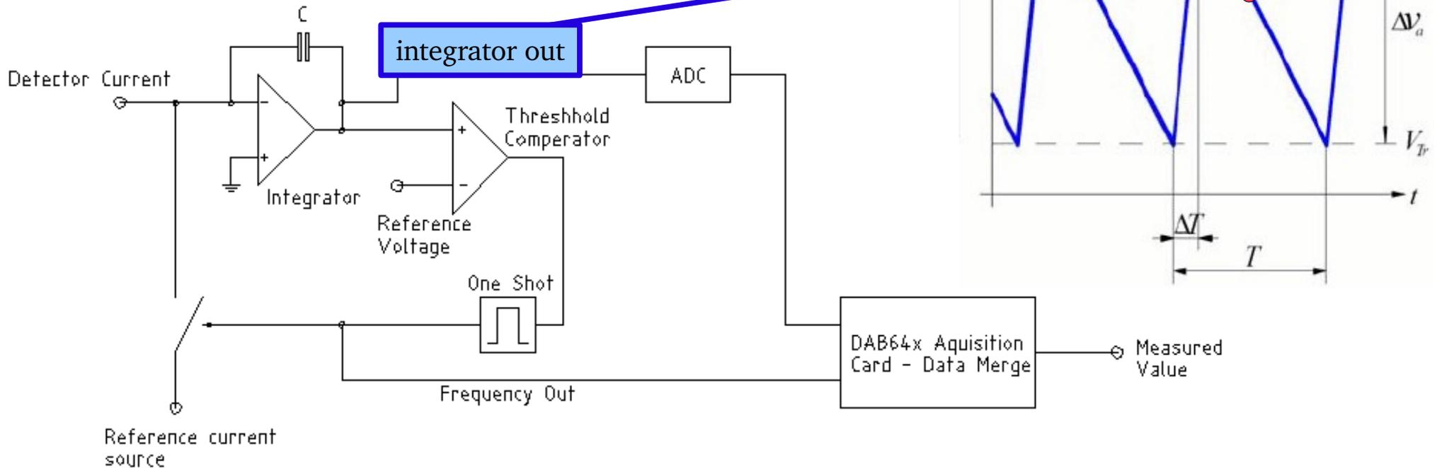
Principle: after reset: C is discharged with detector current.
