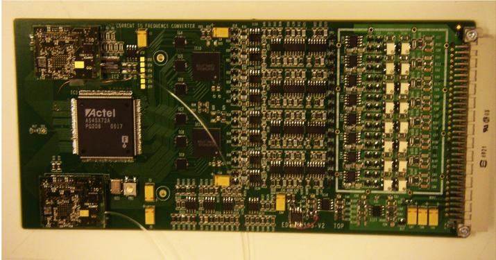
Tunnelcard with current to frequency converter from LHC Beam Monitoring Group (Dehning, Effinger)
