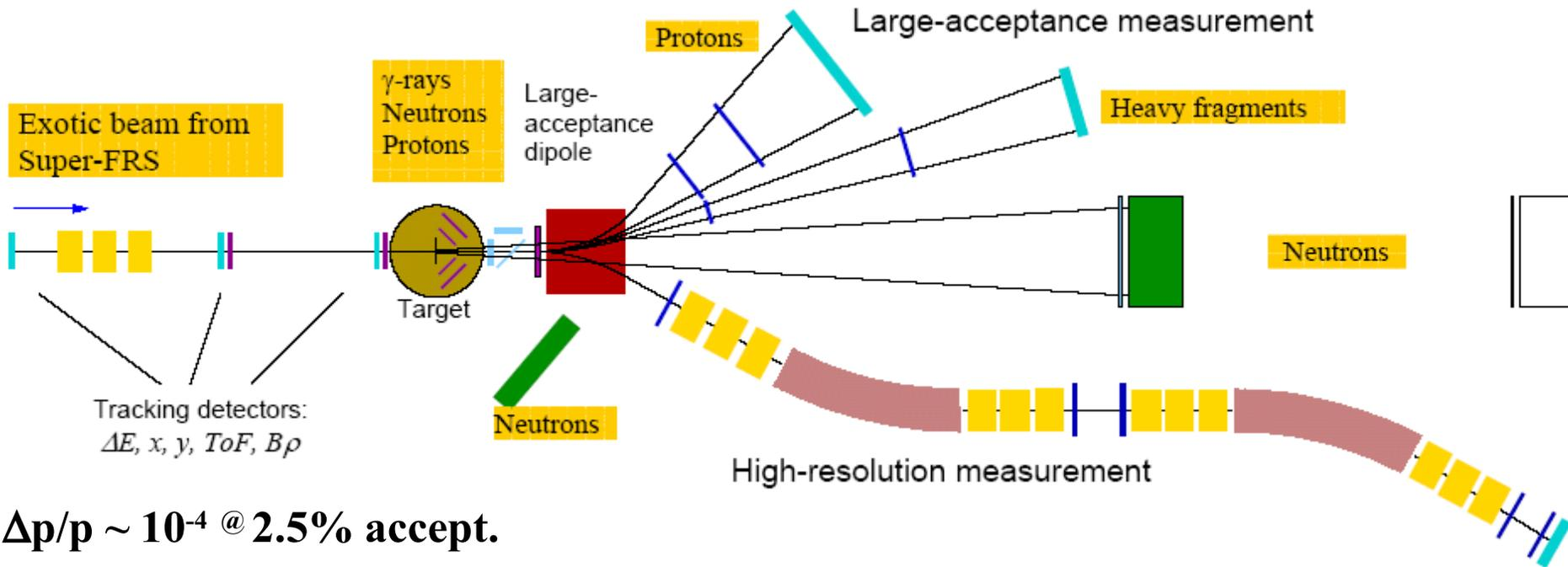
Measurement of all kinematic variables in a HI reaction
