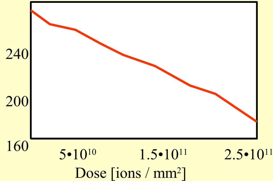
20% signal loss after  $10^{13}$  ions/ $\text{cm}^2$  ( $^{16}\text{O}$ , 120MeV)
