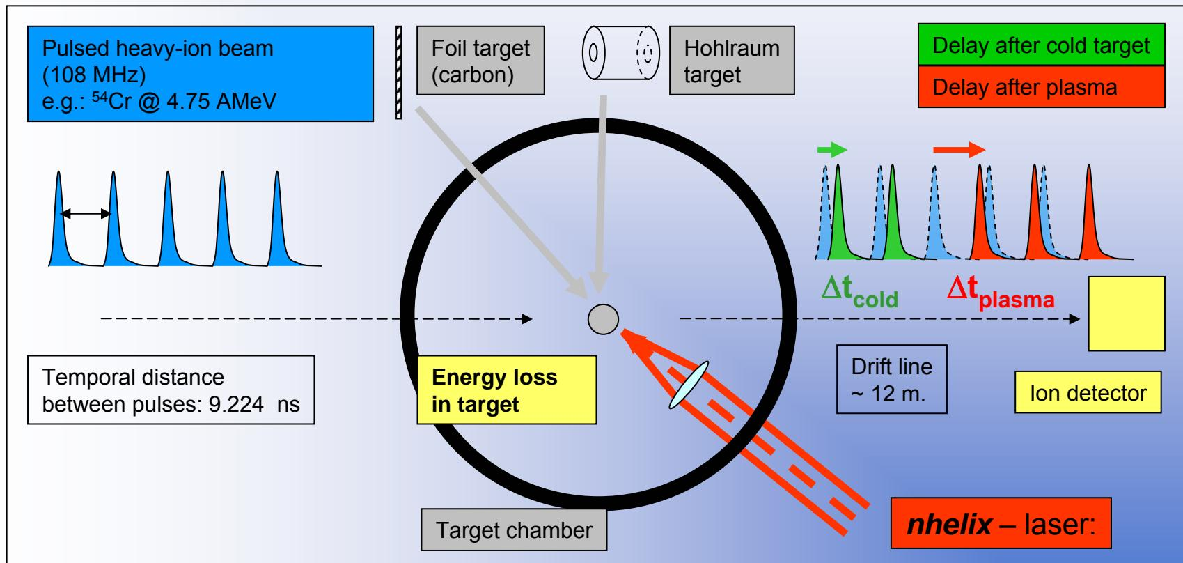
$\Delta t_{\text{plasma}} - \Delta t_{\text{cold}} \Rightarrow$  enhanced energy loss in plasma,  $\Delta E_{\text{plasma}} - \Delta E_{\text{cold}}$ .
