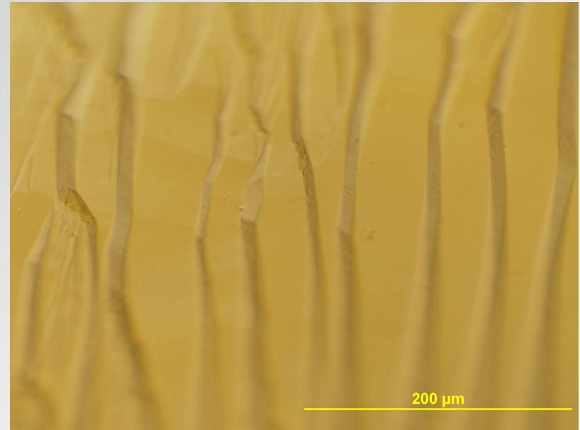
Result of step flow after 1 mm film growth
