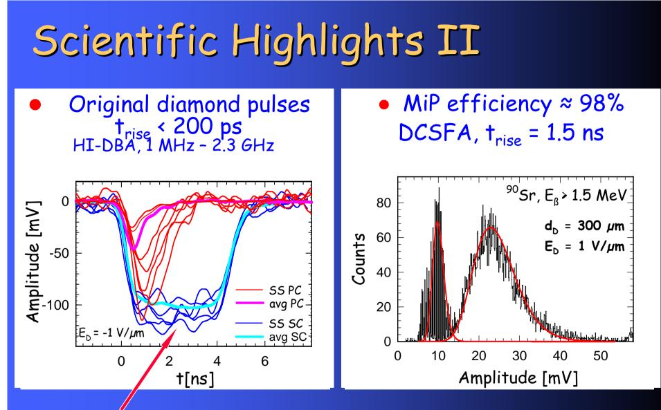
Complete charge collection and fast drift:  $v_{drift} \approx 100 \ \mu m/ns$  $Q_c = 1/R^* \int U(t) dt$
