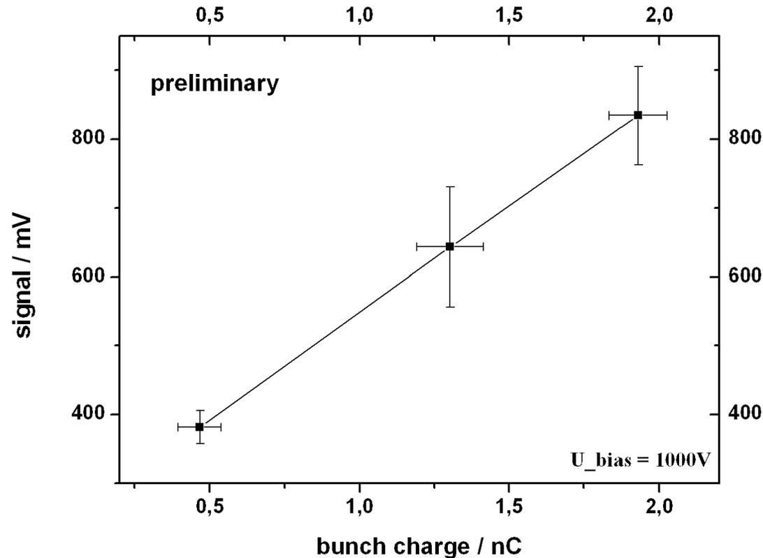
Signals were measured with an RD42 strip-detector. The thickness was approximately  $1100\mu\text{m}$ .
