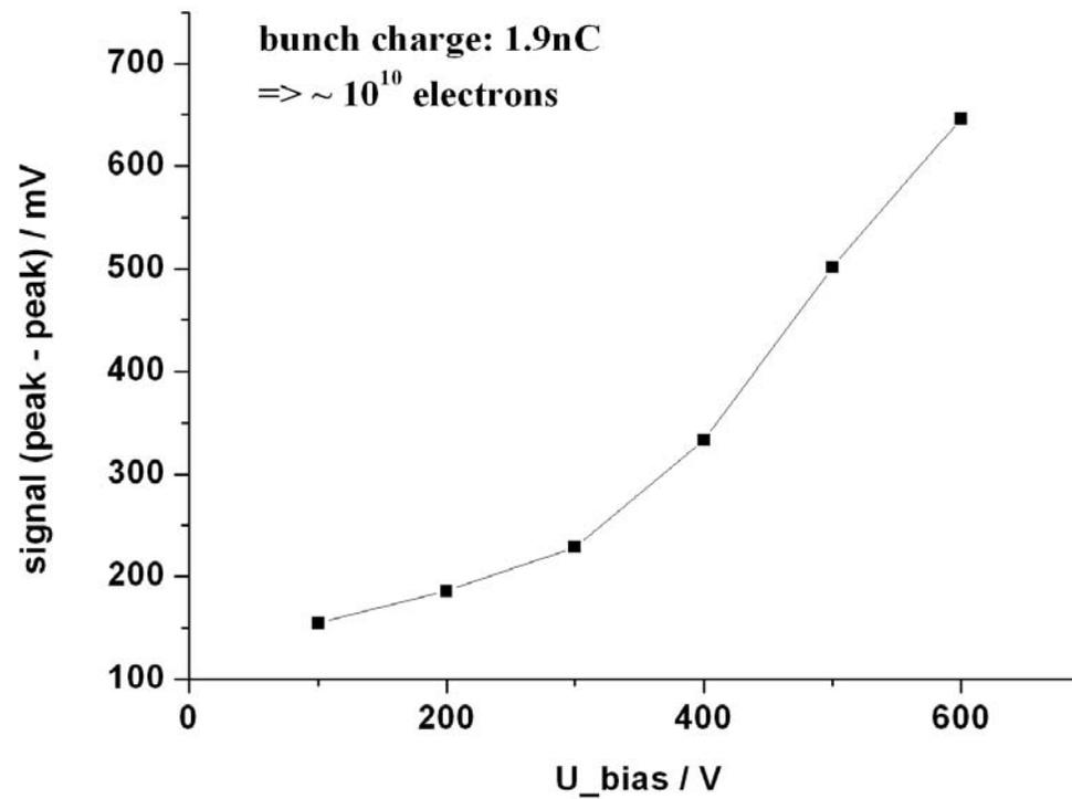
The RD42-strip-detector was used for this measurement. Unfortunately the highvoltage cables did not work properly with voltages higher than 600V.
