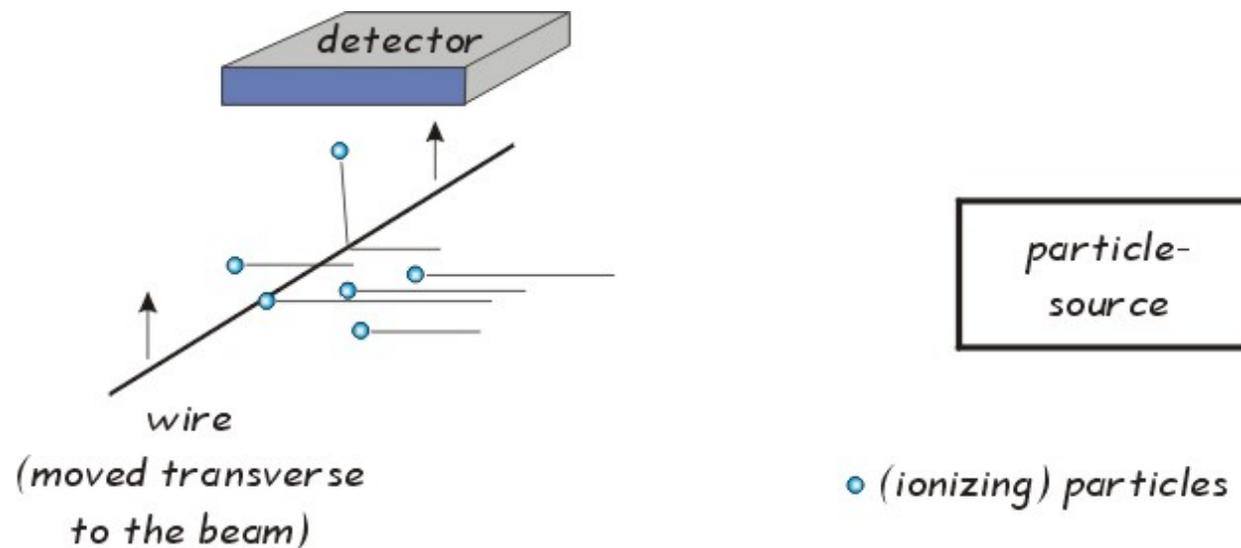
A very thin wire is moved through the beam. From the number of particles scattered into the detector, one can calculate the intensity of the beam at the position of the wire.
