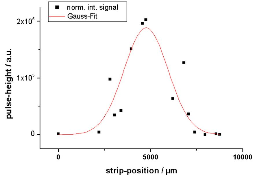
Signals were measured with a 4-channel-oscilloscope and so this profile was measured with a few bunches. Estimating the bunch-width results in a value, which is a little higher than the one estimated with a scintillator.
