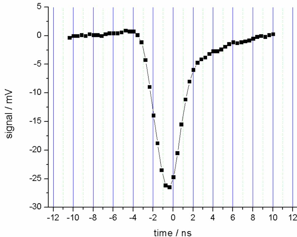
This signal was taken at the proton - cyclotron of the FZK (ForschungsZentrum Karlsruhe), where a pulse is delivered every 38 ns.
