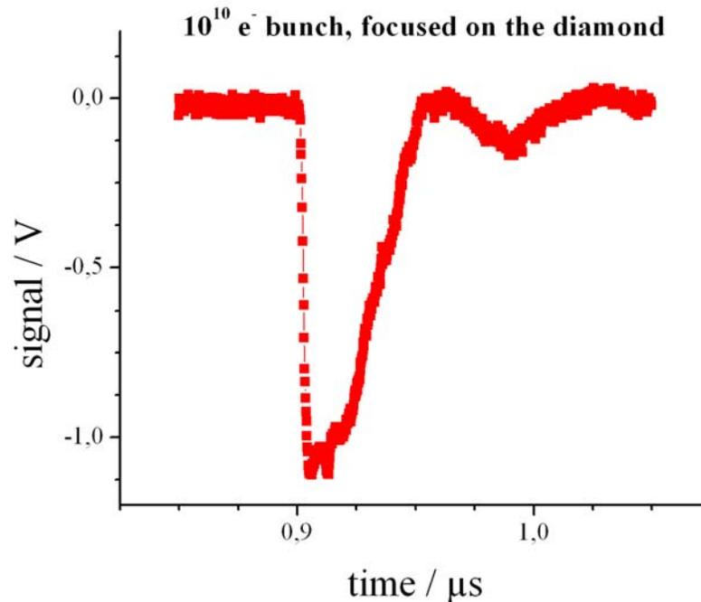
Typical signal of a diamond generated by an electron bunch at the Tesla Test Facility. The diamond was 250 $\mu$ m thick with a circular aluminium pad of 7mm in diameter.
